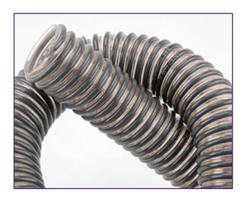
Medium Wall Polyurethane ducting reinforced with a antishock rigid PVC helix. Corrugated outer with a perfectly smooth bore for optimised flow characteristics. Wall thickness from 0.8mm to 1.0mm.
