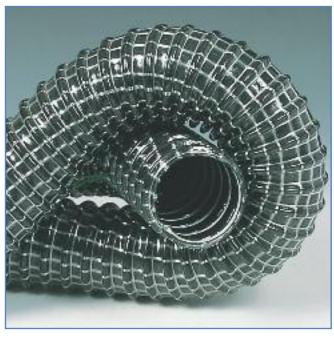
**Construction**: A double ply wall of plasticised PVC encapsulating axial and helical re-inforcing Yarns supported by a PVC coated spring steel Helix.
